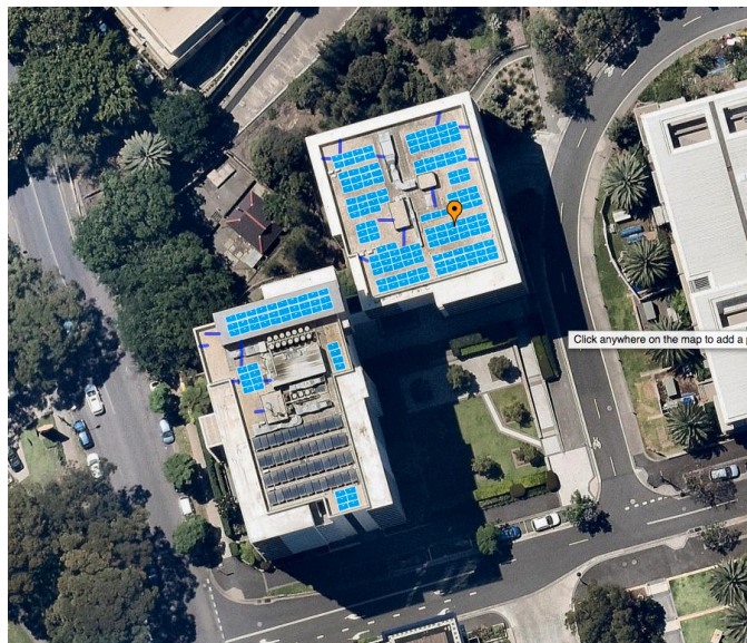
Figure 11 – Example “Full Roof” PV system
